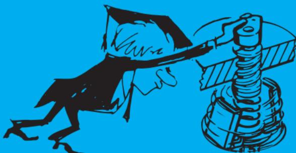
When the cockpit control is pulled back, the governor control lever and shaft turn in the opposite direction, relaxing compression on the spring. This reduces the speed necessary for the flyweights to move the pilot valve and produces a lower RPM setting.
